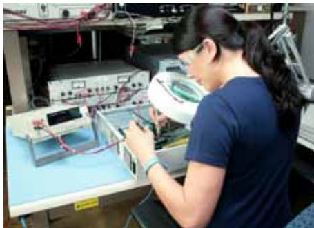
Figure 1. Smaller UPS models are usually sent to a repair facility.
