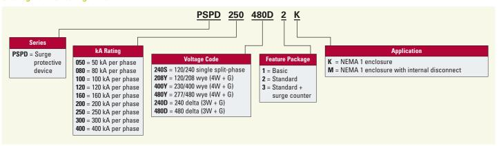
**Example:** PSPD250480D2K = SPD Series, 250 kA per phase, 480D voltage, standard feature package, housed in NEMA 1 enclosure
